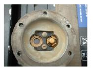
Remove the in and out fuel pipes the cap and filter. Remove the 6 retaining screws, lift top off. Rotate the diaphragm and remove. Above the 3 pieces separated. The pump base, the diaphragm and the top non-returns, all looked in reasonable condition so have been kept for emergency repair!
